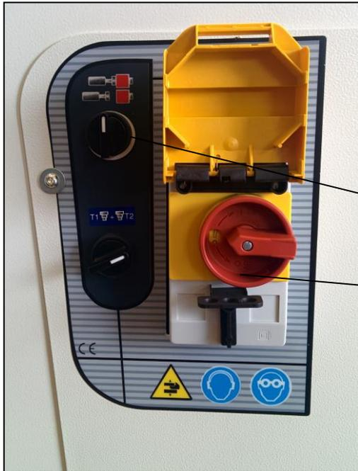
To turn on the copy router the switch must be activated (A)
