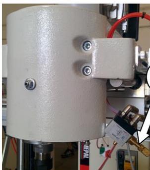
Periodically replace the cooling lubricant that is contained in the relevant tank (B). Failure to observe this rule will invariably cause machining to be rougher and the mills to wear out more rapidly. In the event that increased tool lubrication is required, use the regulator (C) on the control panel of the router head.
