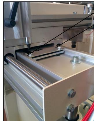
By using the selector button as shown in the detail (B), the tracer points are activated.
